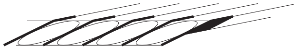
Figure 7.12: The black lines and black surface visualize the location of a highly resistive coating at the thin edge of the cable.
